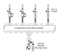
undesirable. If condensate outflow is to be used to warm or freeze protect a small device, you must provide several feet of bare tubing ahead of (upstream of) the valve to provide the condensate. A #20 mesh strainer is recommended to use with all port sizes.
