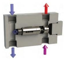
The thermal actuator will monitor the inlet flow and divert the fluid based on temperature. Cooler fluid will go through the bypass of the valve. Hot fluid will activate the thermal actuator, causing the internal cartridge to close and forcing the fluid through the system cooler.
