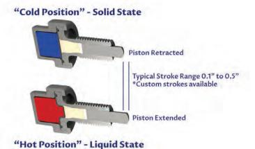
Our Thermoloid® material operates at temperatures ranging from 15°F to 300°F (-9.44°C to 149°C). Because of the gradual transition from solid to liquid of this Thermoloid® material, these valves act more like modulating valves rather than quick opening/closing valves. Our Direct Acting Valves are designed to be open when the actuator is in the "cold position" while Reverse Acting Valves are open in the "hot position".
