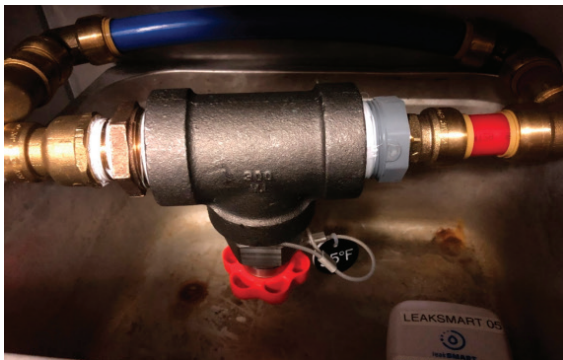
Figure 1. GURU® DL 2.1 Low Temp Test Set Up
